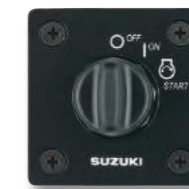
IGNITION SWITCH PANEL SINGLE IGNITION
