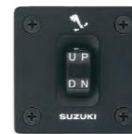
PTT SWITCH PANEL
