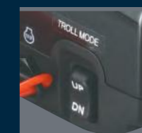
Troll mode switch activates Suzuki Troll Mode System and controls RPM from idling engine speed up to 1200rpm at every 50rpm
